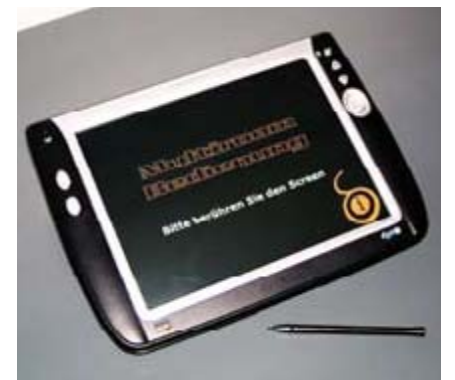
Radio touch panel with embedded windows
