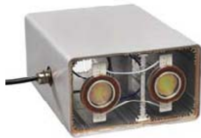
Prototype for underwater loudspeakers
